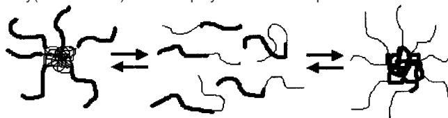
Scheme 2. Simplified Model of the Changing Association of Poly(NIPA- b -SPP) Block Copolymers with Temperature
